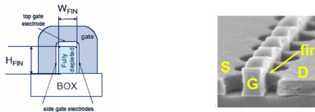
Figure 17. Cross-section of an advanced FinFET.
