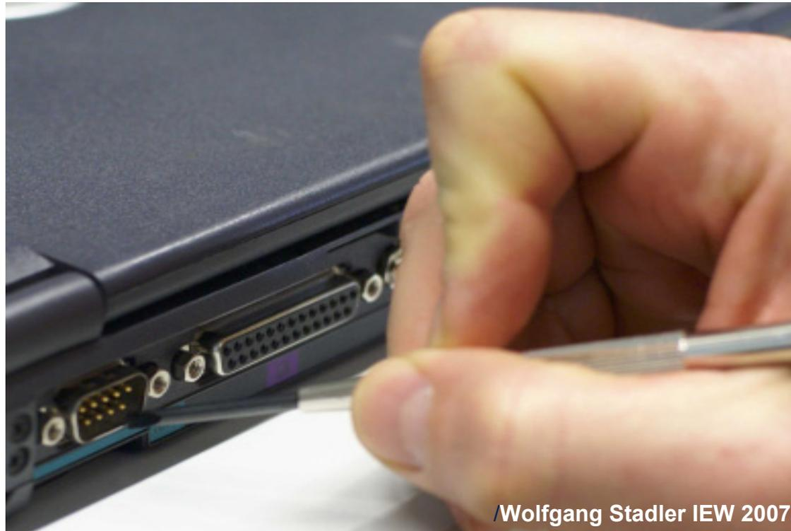
Discharges from a handheld metallic tool to a system (outside an EPA) are tested by system level ESD (e.g. IEC 61000-4-2)
